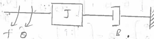
$$\text{Torque balance eqn} \quad T = J \frac{d^2\theta}{dt^2} + B \frac{d\theta}{dt} \rightarrow \textcircled{3}$$
