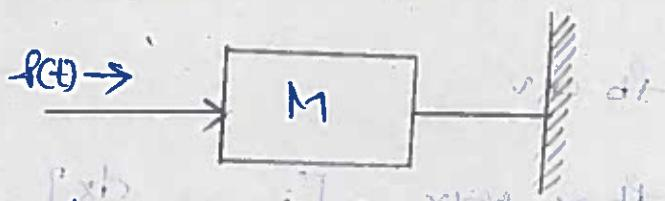
Consider an ideal mass element as shown in figure, which has negligible friction and spring let a force be applied on it. The mass will offer an opposing force which is proportional to acceleration of the body
